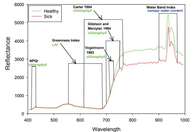
Figure 3. The full visible and NIR spectrum are not required to predict ash decline. Here we used six known plant stress indices that are sensitive to changes in chlorophyll content, function or canopy water content. Such indices generally pair a stress sensitive wavelength, with an insensitive wavelength to account for differences in shading, view angle, or background interferences.
