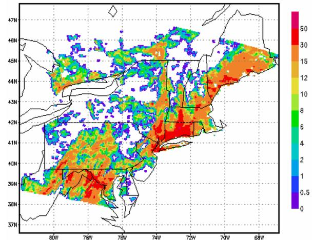
Figure 7. Positive linear regression correlation coefficients ( $\times 100$ ) of simulated HI and near-surface TKE at 20Z for the period of 1 March 2003 – 18 July 2003 (only over land). Note the irregular contour intervals.
