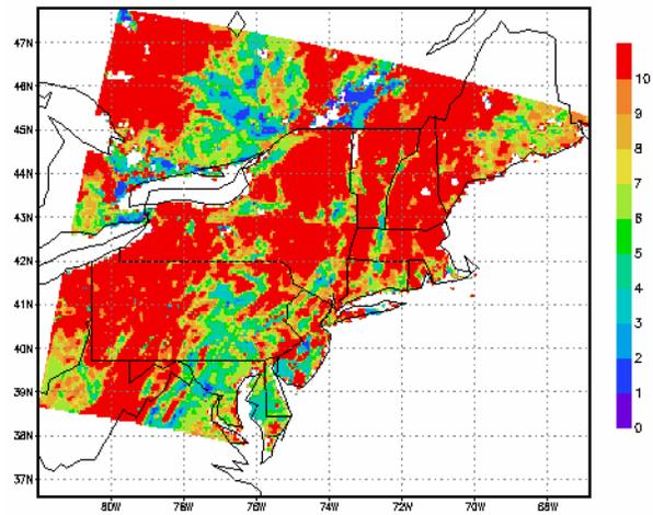
Figure 6. Same as Figure 5 except for simulated frequency (%) of near-surface TKE values greater than  $4 \text{ m}^2 \text{ s}^{-2}$ .
