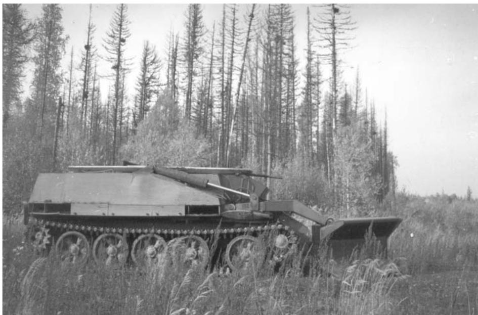
*Figure 3.* Special-purpose bulldozer for knocking down snags and constructing firelines.
