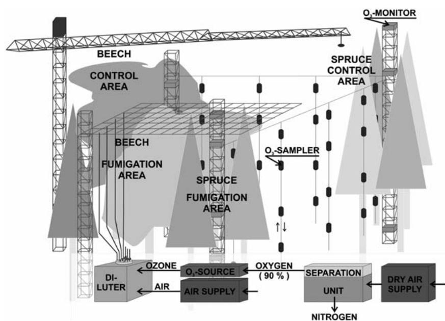
**Fig. 6** The experimental setup of the KROFEX experiment, located near Munich, Germany. Ozone is produced by a commercial ozone generator fed with 90% oxygen, which is separated on site from dry purified air. Diluted ozone is pumped to the fumigated canopy volume (approx. 2000 m<sup>3</sup>) by means of 117 PTFE tubes and distributed via approx. 6000 calibrated outlets. Ozone monitoring is done continuously by 8 online monitors and 100 passive samplers replaced at weekly intervals.
