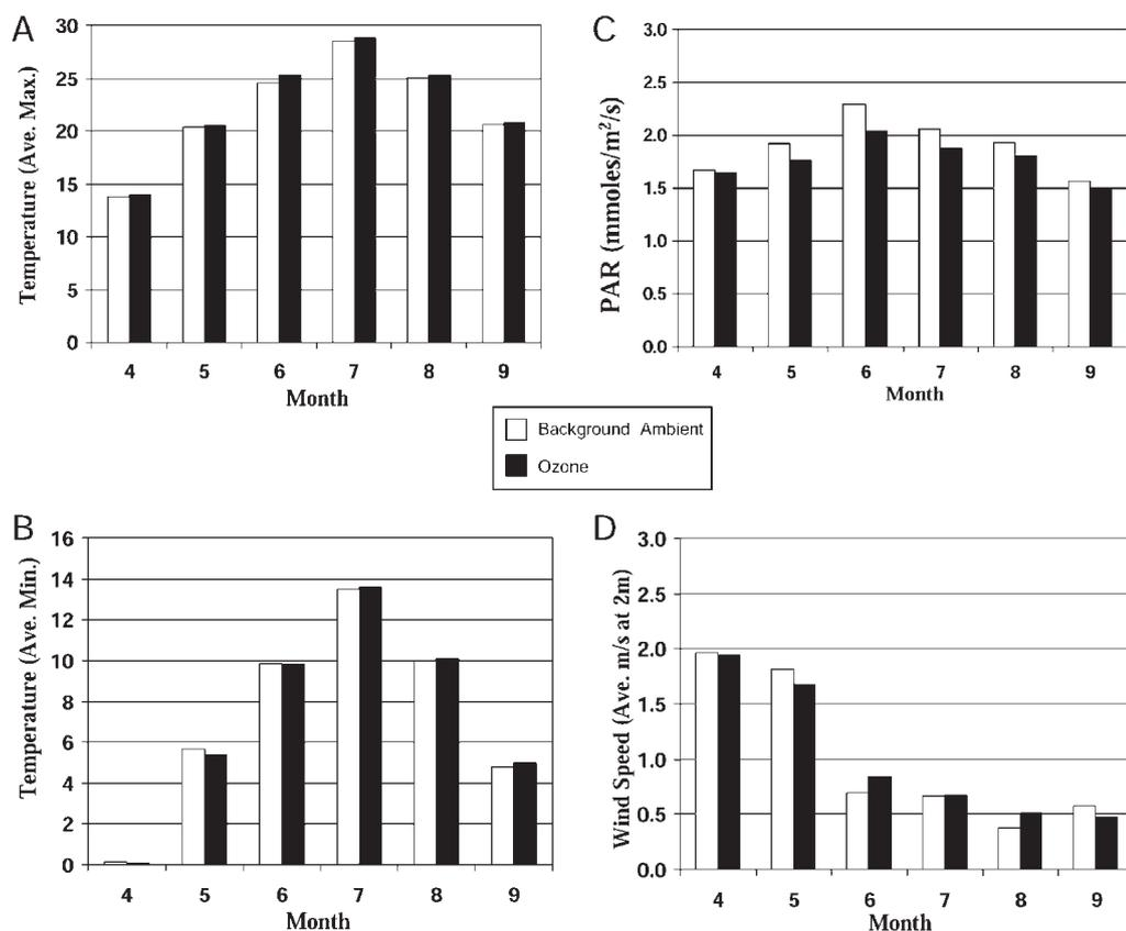
**Fig. 2** The Aspen FACE experimental rings have had minimal impact on micrometeorology, as shown in these comparisons for background ambient conditions and an O<sub>3</sub> ring for maximum (A) and minimum air temperature (B), PAR (C), and wind speed (D). All values were taken in the mid-canopy height of the aspen section in 1999 and are monthly averages.
