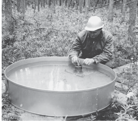
FIGURE 2.14 Hydrological technician Clarence Hawkinson measuring water levels in the S2 evaporation pan during August 1963. (Photo courtesy of D.H. Boelter, USDA Forest Service, Grand Rapids, MN.)
