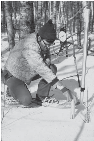
FIGURE 2.4 Hydrological technician Art Elling using a Mount Rose snow tube to measure snow depth and water equivalent along the S1 upland snowcourse. The hanging scale is used to weigh the snow tube to determine snow water equivalent. (Photo courtesy of unknown photographer, USDA Forest Service, Grand Rapids, MN.)
