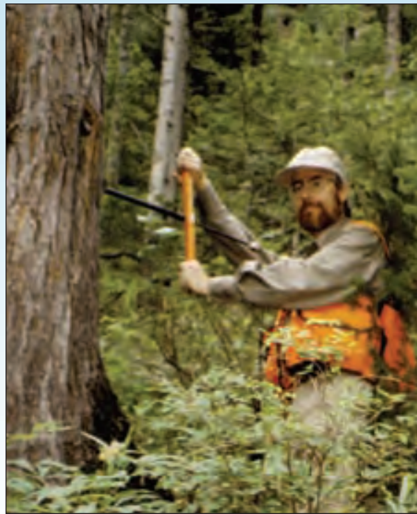
Figure 2. Collecting a sample of tree rings with an increment borer in southern Siberia.
