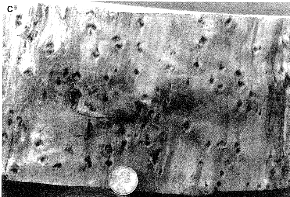
Figure 12.—Appearance of birdseye on the outer surface of the xylem. Relatively small (a), medium (b), and large (c) birdseyes (note penny for scale).
