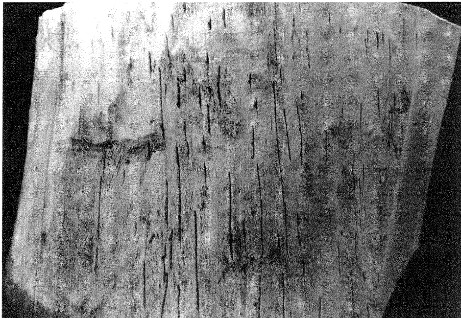
Figure 4.—“Fingernail” or “thumbnail” birdseye in sugar maple, with a few “normal” birdseyes scattered among the fingernails.
