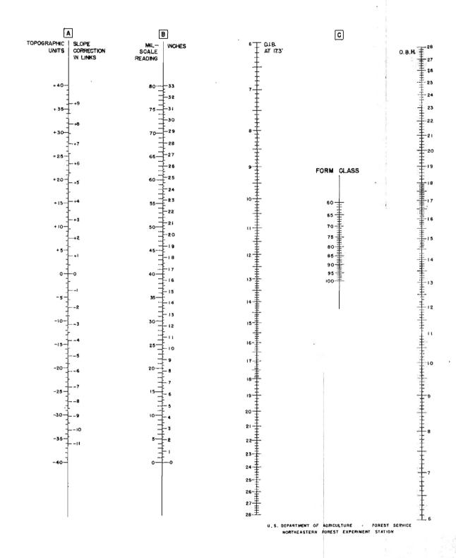
FIGURE 5.—Alinement charts used in estimating form class with the aid of mil-scale binoculars.
